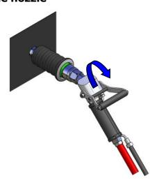
5. Pull back on the black sleeve to disconnect the nozzle from the receptacle
