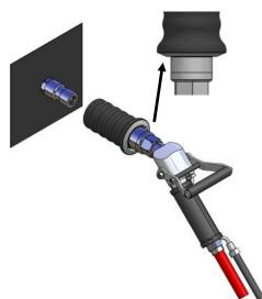
2. When coupled the nozzle will click into position and the green indication sleeve is visible
