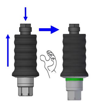
2. Remove green sleeve retaining ring and discard.
