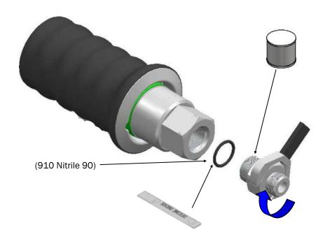
Torque the nozzle to 90Nm when tightening
