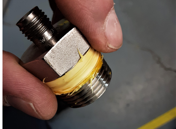
Figure 8. Thread after 5 installations with correctly applied PTFE tape.
