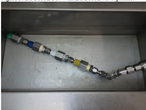
Figure 5. Fittings tested for leakage in water bath.
