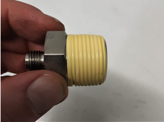
Figure 7. Tape applied to fitting ensuring coverage of all threads.
