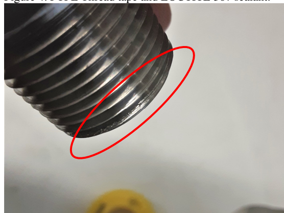
Figure 6. Galling on the first thread (circled) of the fitting after testing with gas-rated PTFE tape. This thread was not covered by the tape.
