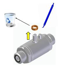
4. Remove face O—rings from valve cap and body. Discard O—rings.
