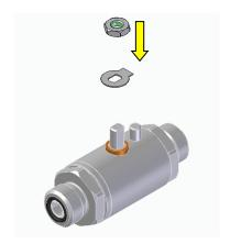
10. Using pliers bend the lock tab upwards so that it is tight against the nut.
