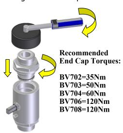
8. Install the handle, washer and nut.
